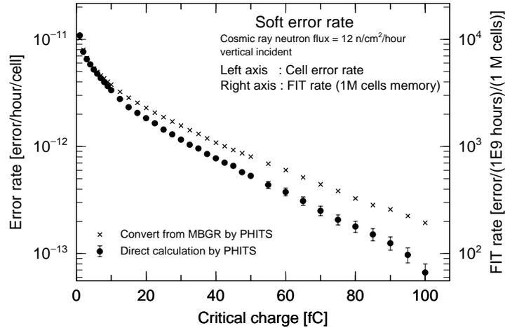
Figure 8: Soft error rate as a function of the critical charge. The unit of left axis is the error rate of a memory cell. The unit of right axis is the FIT rate [error/10<sup>9</sup> h/device] of a device with 1 M cells.
