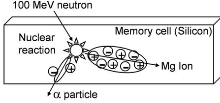
Figure 1: An image view of a neutron-induced soft error process.
