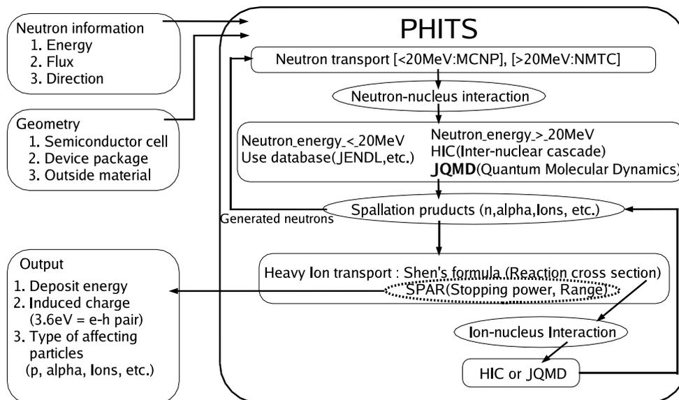
Figure 3: The concept flow chart of the soft error simulation by PHITS.
