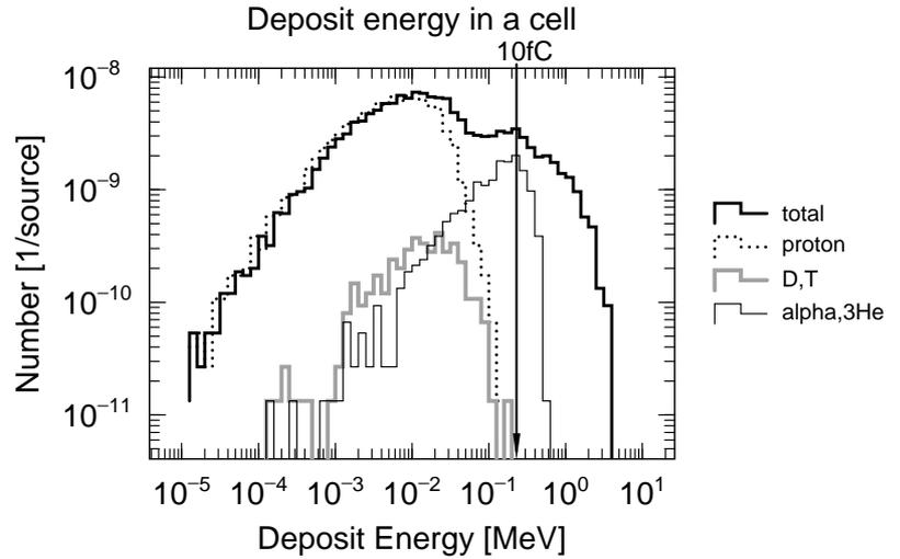
Figure 7: Deposit energy distribution in the sensitive region of a SRAM cell.
