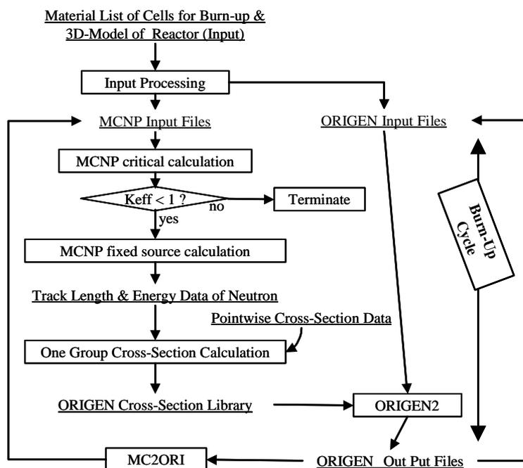
Fig. 1. Flow chart of burn-up calculation
