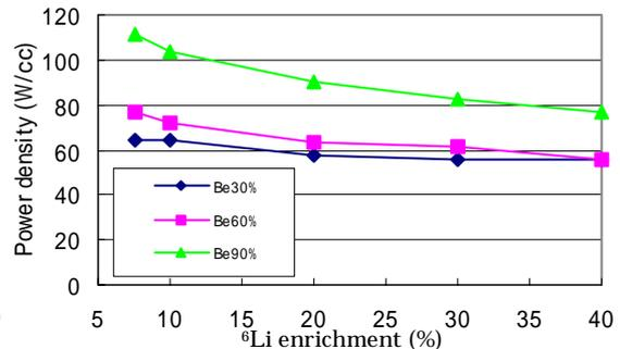
Fig. 4 Power density of WC blanket at BOC
