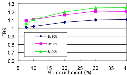
Fig. 3 TBR for WC blanket at BOC
