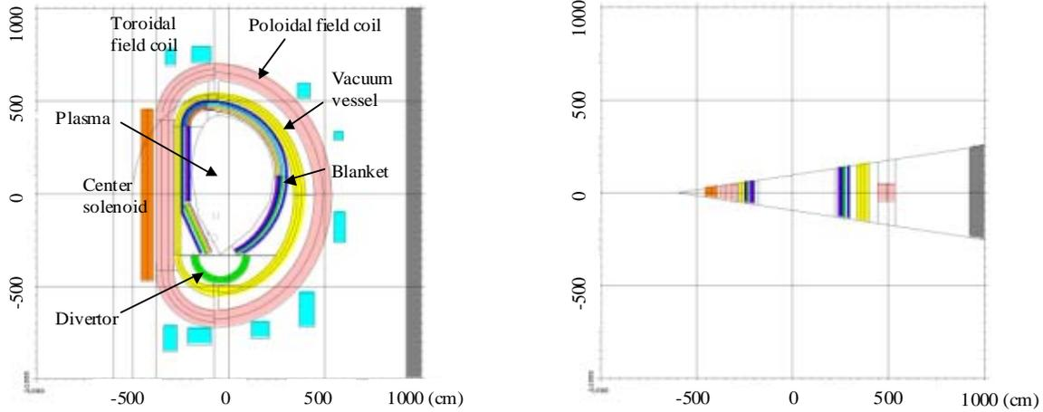
Fig. 2. Vertical (left) and horizontal (right) cross-sections of calculation model
