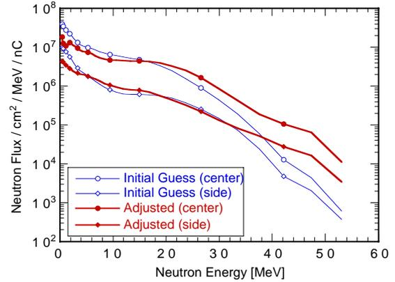
Fig. 5 The initial guess and adjusted neutron flux spectra for the d-Li neutron field.
