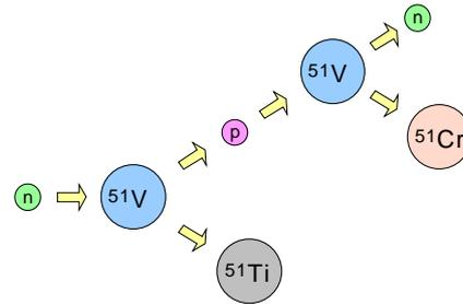
Fig. 7 Sequential charged particle reaction.
