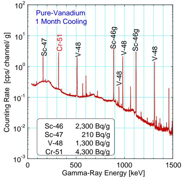
Fig. 6 Gamma-ray spectrum for the pure-vanadium sample measured after 1 month cooling.
