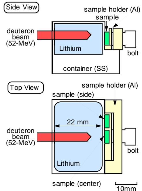
Fig. 1 The lithium-target and sample arrangement.
