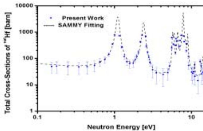
**FIGURE 2.** Comparison of the measured total cross sections of natural Hf with the predicted ones from the SAMMY fitting.
