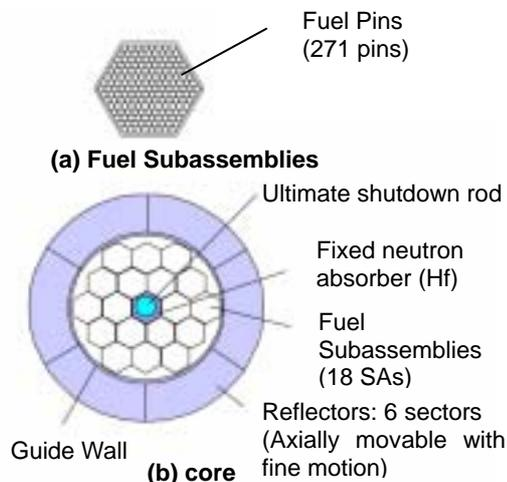
Fig. 2 Design of the Non-refueling core
