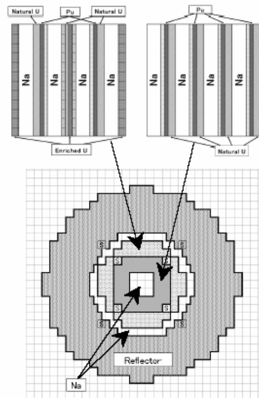
Fig. 3 Cross sectional view of the experimental core (FCA XXIII core)
