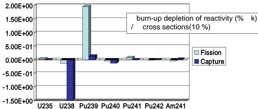
Fig. 6 Sensitivity coefficients of burn-up depletion reactivity
