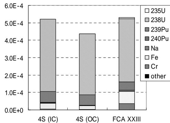
Fig. 5 Nuclide-wise component of SVS (conversion ratio)
